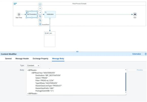
2. Use the integration flow ID to run the integration flow with a Process Direct Call between a Request Reply and a Receiver.
