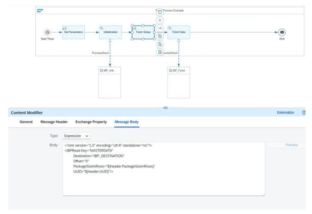
2. Call the integration flow with the Process Direct Call using the ID of the integration flow.
