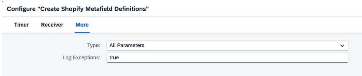
Figure 4.3.2.2 Configuring the Integration Flow’s More Configuration
