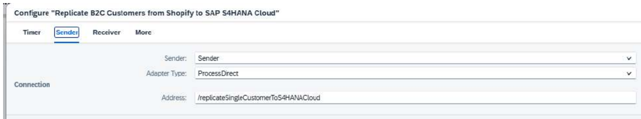
Figure 4.3.6.2 Configuring the Replicate B2C Customers from Shopify to SAP S/4HANA Cloud Public Edition Integration Flow’s Sender
