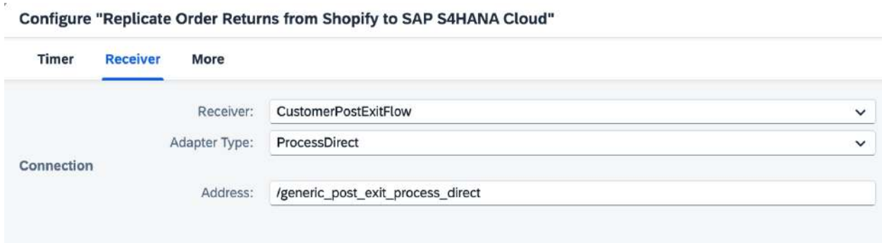
Figure 4.3.9.6 Configuring the Integration Flow's CustomerPostExitFlow Receiver
