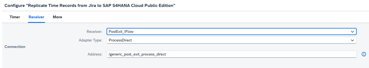
Figure 4.3.6.2.4 Configuring Replicate Time Records from Jira to SAP S4HANA Cloud Public Edition Flow Receiver PreExit_IFlow
